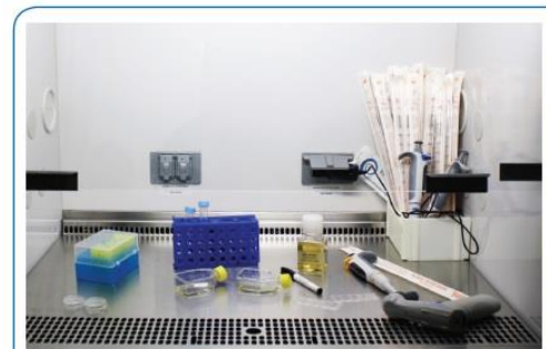
Figure 3: Cell culture hood and standard equipment.
