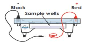
3.c) Fill the electrophoresis apparatus chamber with **300 ml of Electrophoresis Buffer 1 X.** *The electrophoresis buffer can be used for 2 electrophoresis experiments, once finished the electrophoresis you can store the buffer used, in a packing different to the supplied, to use it in a new electroforesis.*
