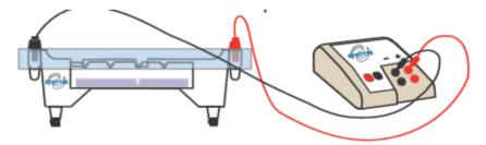
3.b) Set the power source at the required voltage and conduct electrophoresis for **75 (30 min)** - **150 (20 min) volts.** Check that you see the current flowing properly - you should see bubbles forming on the two platinum electrodes.
