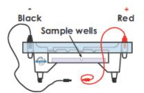
3.c) Fill the electrophoresis chamber with **300 ml of 1x electrophoresis buffer**. *The electrophoresis buffer can be used for 2 electrophoresis practice. Once the electrophoresis is finished, store this used buffer in a different container; don't mix a electrophoresis buffer new with one used buffer.*
